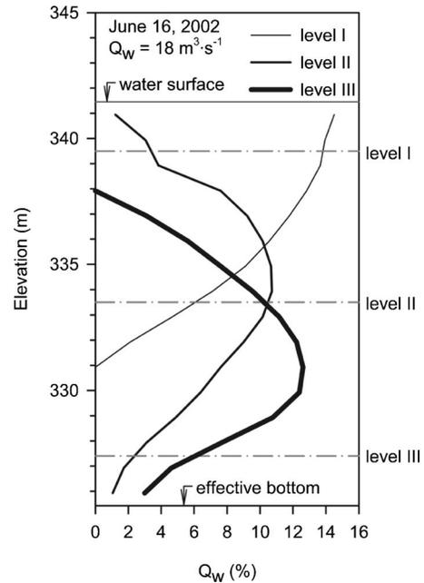
**Fig. 3.** Model simulations of vertical contributions to withdrawal flow ( $Q_w$ ) for conditions of June 16, 2002, for three intakes (centerline positions shown), operating separately
