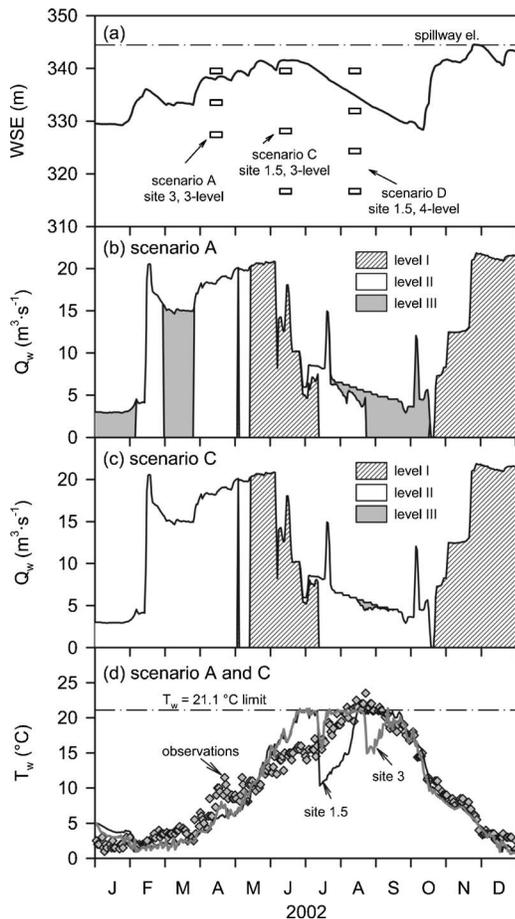
**Fig. 5.** Time series for Case 1 (conditions of 2002): (a) WSE, with vertical positions of intakes presented for multilevel intake scenarios; (b)  $Q_w$  (observed) and simulated apportionments for intake levels of Scenario A; (c)  $Q_w$  (observed) and simulated apportionments for intake levels of Scenario C; and (d)  $T_w$ , observations and model predictions for Scenarios A and C
