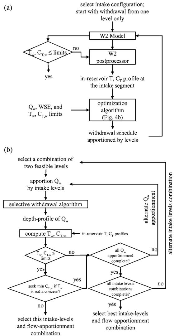
**Fig. 4.** Optimization for operation of multilevel intake facility: (a) linkage of two-dimensional water quality model and optimization algorithm; (b) heuristic optimization algorithm for blending of withdrawals from multiple intakes to meet  $T_w$  goal and minimize  $C_{T,w}$
