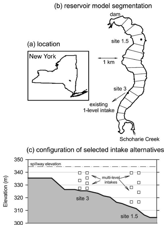
**Fig. 1.** Schoharie Reservoir: (a) location within New York; (b) map with locations of Schoharie Creek inflow, existing water supply intake, potential sites for multilevel intakes (1.5 and 3), and longitudinal model segments; and (c) vertical positions for four intake scenarios (Table 1)
