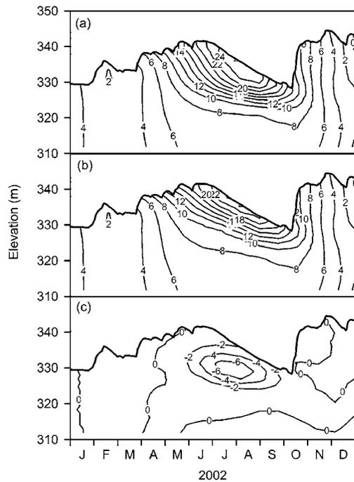
**Fig. 8.** Simulated isotherms for Site 1.5 for Case 1 (conditions of 2002): (a) for existing single level intake; (b) for multilevel intake Scenario A; and (c) residuals for existing single level intake and Scenario A (negative values depict temperature decreases from existing intake conditions)
