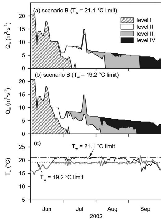
**Fig. 6.** Time series for Case 1, for conditions of June–September 2002: (a)  $Q_w$  (observed) and simulated apportionments for intakes of Scenario B, for a  $T_w$  limit of  $21.1^\circ\text{C}$ ; (b)  $Q_w$  (observed) and simulated apportionments for intakes of Scenario B, for a  $T_w$  limit of  $19.2^\circ\text{C}$ ; and (c) model predictions of  $T_w$  for Scenario B
