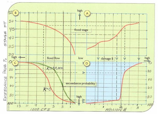
The figure above shows the calculation of the probability of annual flood damage (quadrant D) derived from the expected stage-damage function (quadrant A), based on the stage-flow relationship (B) for the flood with expected probability of exceeding an annual peak flow (C).
