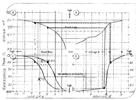
A flood control project with storage of 50,000 Ac-ft is planned on the Great Plains River to reduce the flood damages through Plainville. The frequency and damage data were compiled as shown above.
