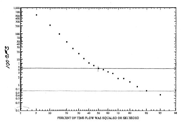
We need to determine the potential for hydropower revenues if we could build a low-head hydropower project at this location where the net Head is 10 ft. for a wide range of turbine releases. We estimate plant efficiency to be about 70%.
