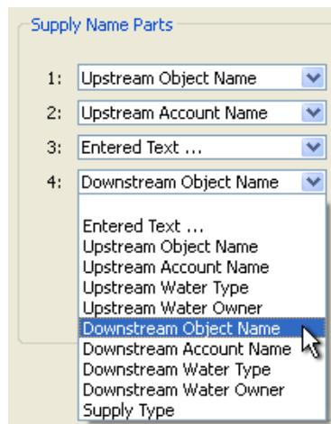
The user can insert, append and remove Supply Name Parts (rows) using the Plus and Minus icon buttons. Up to 12 parts can be defined:
